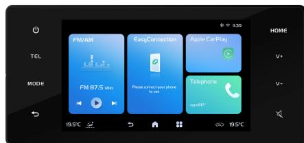
Press and hold the button
