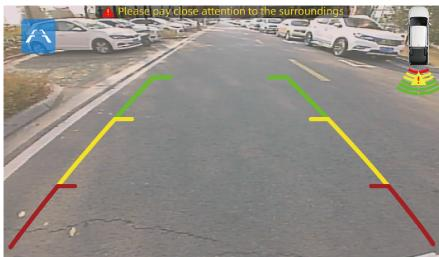
Engage the R gear to enter the RVC screen.
