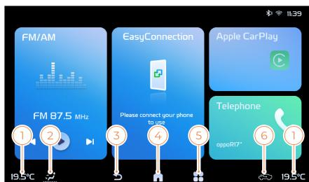
If the A/C settings menu is closed, you can use the toolbar buttons below for quick control:
